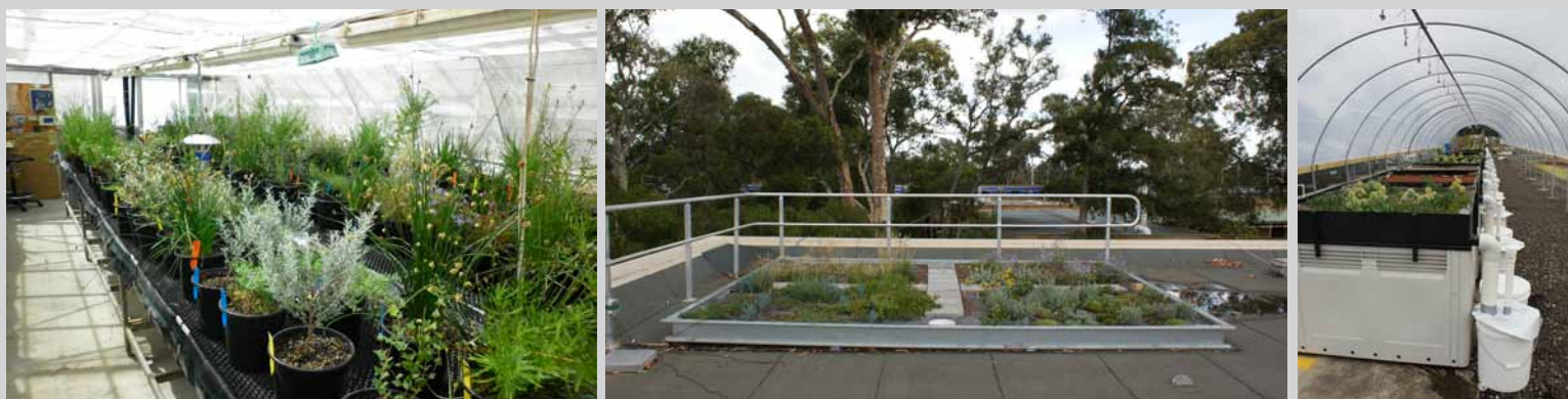
Figure 18. Green roof research at the University of Melbourne includes plant survival experiments in glasshouses and on roofs, and hydrology experiments in controlled environments under cover.
